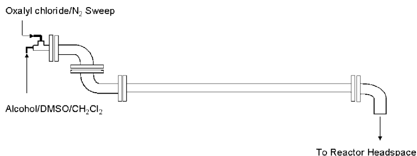
Figure 4. Diagram of pilot-plant in-line reactor.
